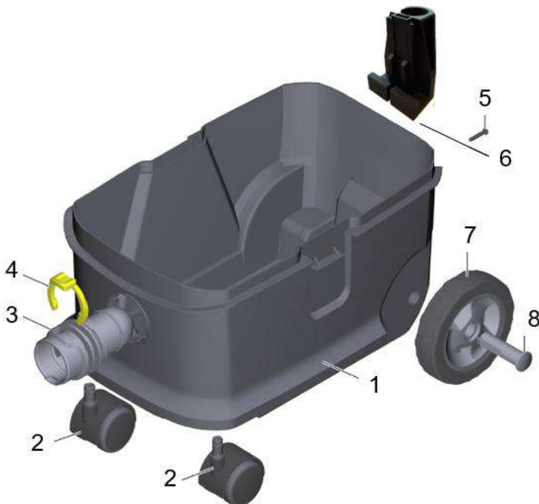
Fig. 3: Explosion drawing of the container
