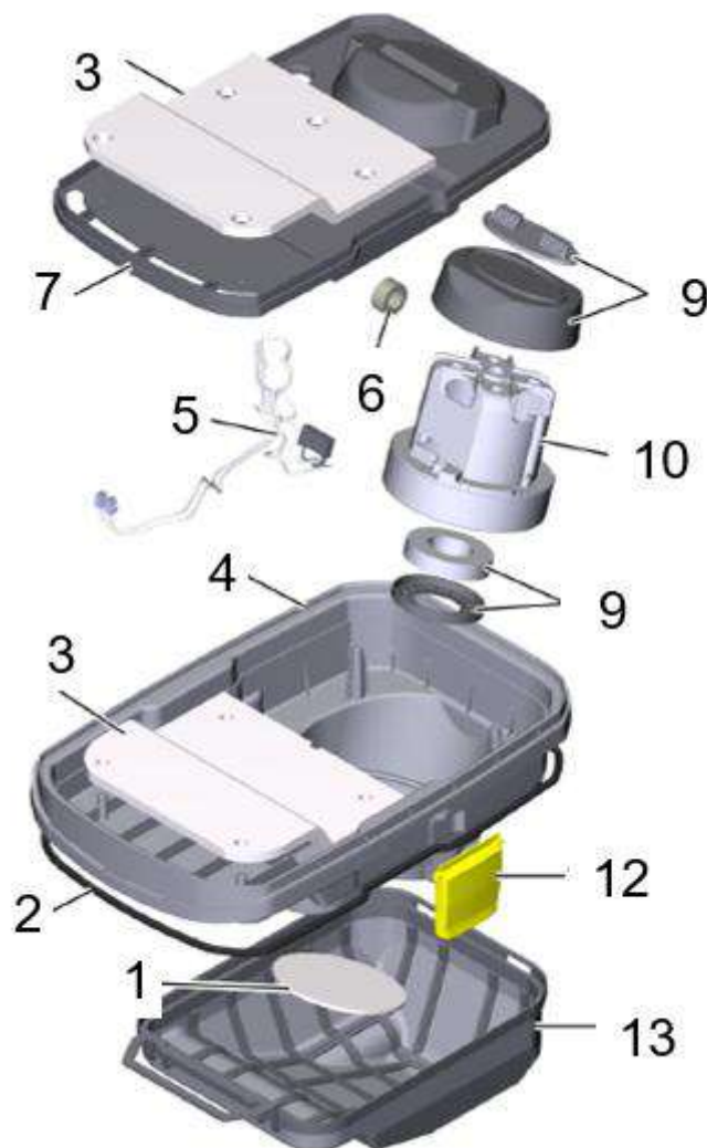
Fig. 2: Explosion drawing the suction turbine
