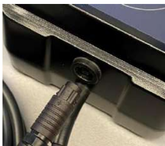
Fig.6 Align white dots and push together
