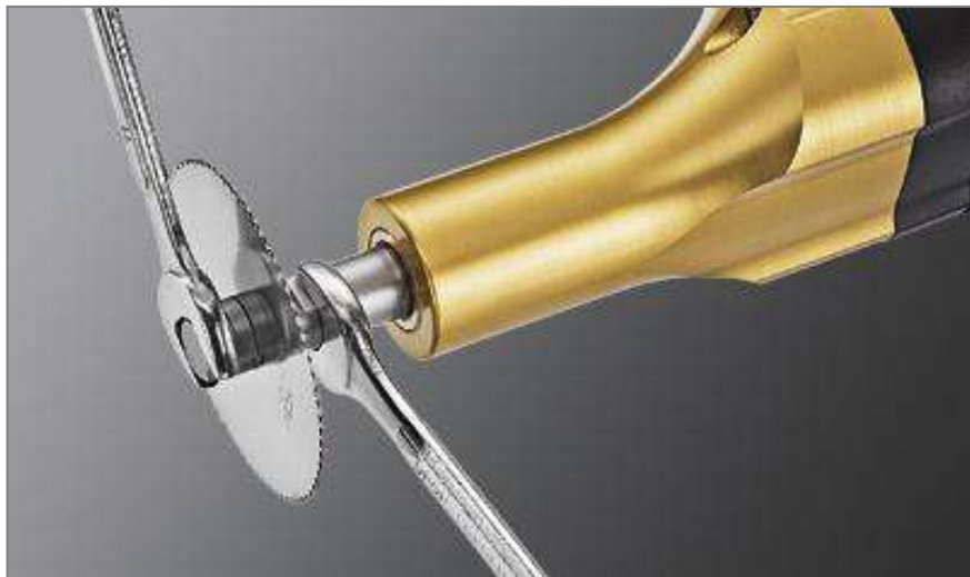
Fig. 1: Releasing the retaining screw
