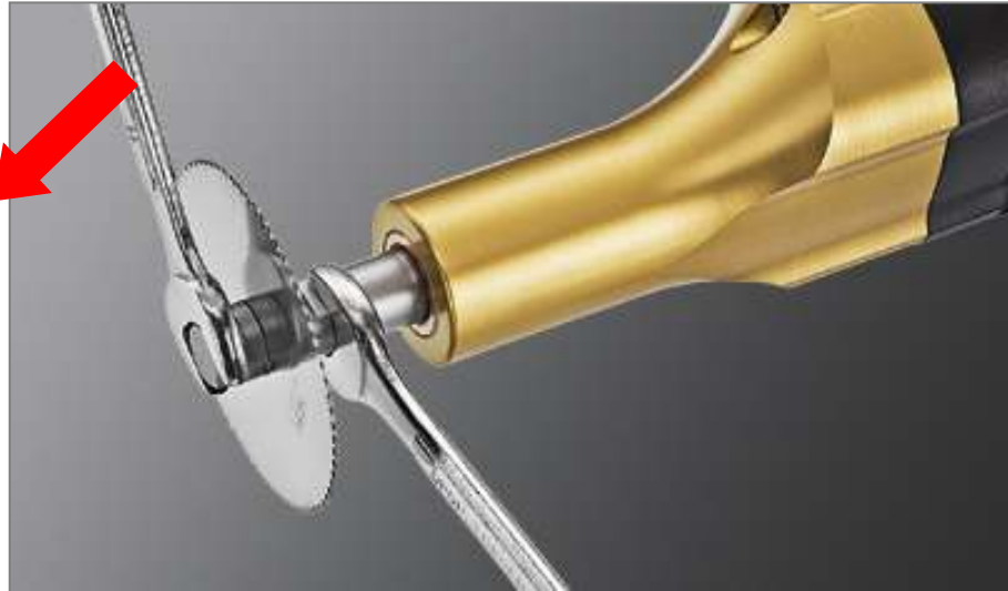
fig. 3 Releasing the retaining screw
