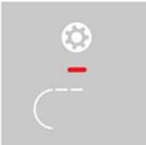
Abbildung 2: CO2 Example of an operating unit fault with 3 illuminated elements → Fault / failure CO2 combi sensor.
